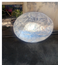
Fig: 2 Aluminium reflector is mounted on parabola
