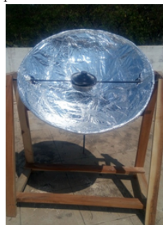
Fig: 3 Parabolic solar cooker
