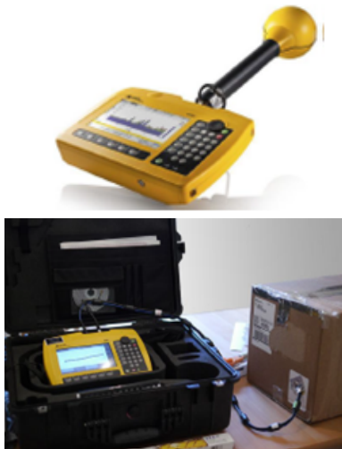
Figure 1.4. Test Setup for SRM-3006 Meter
