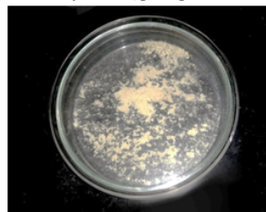
Figure 6: \text{CaCO}_3 powder obtained after filtration
