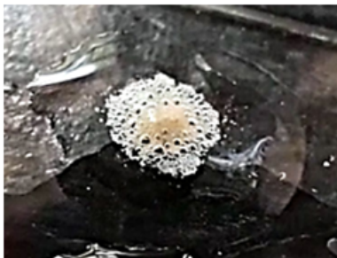
Figure 7: Effervescence seen after treating the obtained precipitate with 2N Hcl.
