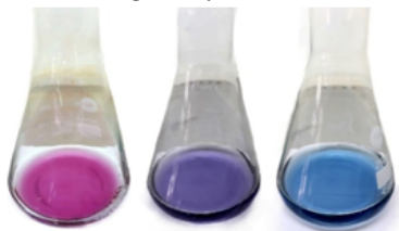
Figure 21: Titration of hard water samples against 0.01M EDTA
