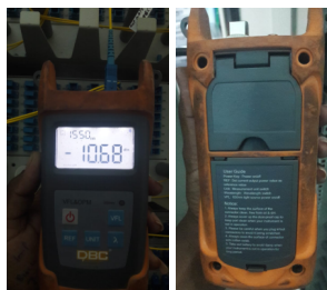
Fig 3: DBC Power meter to monitor the sensor response in decibels (dB)
