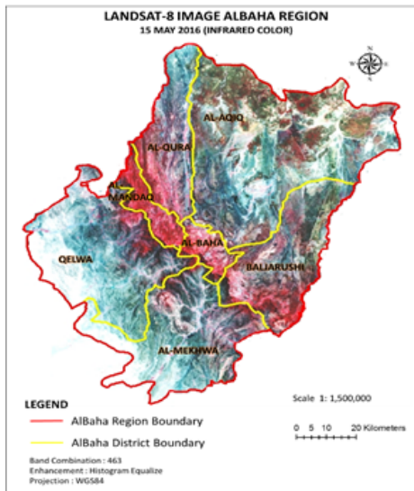
Figure 6 : Vegetation Density Map of Al-Baha Region (Infrared Color). Red color indicates vegetation presence
