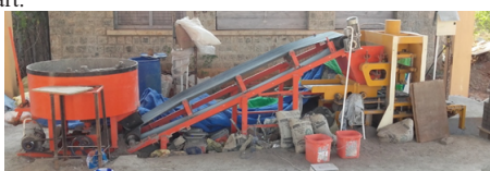
Fig 1: Fly ash bricks casting machine
