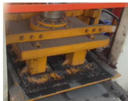
Fig 2: Compressing fly ash bricks with a pressure of 150 Kg/cm²
