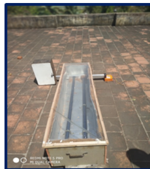
Fig.1 Solar air heater constructed with evacuated tubes.
