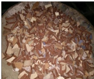
Figure 3.5.1 ceramic tile aggregate
