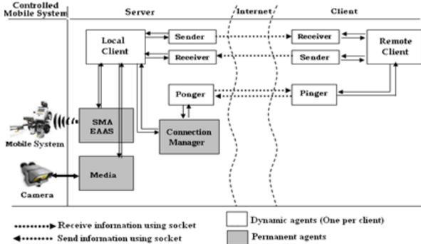
Figure 6. Remote Control Software Architecture Proposed
