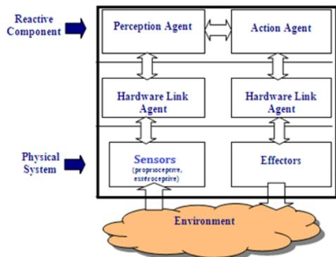
**Figure 5. Reactive Part Of The EAAS Architecture**
