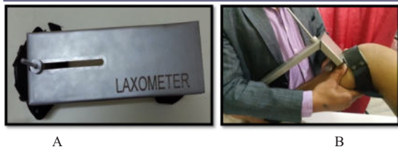
Figure 1 A: Showing Laxometer. B: Showing Lachman test with the help of Laxometer.
