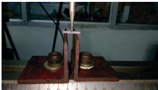
Image 3 : Showing fracture of sample with three point bending test for the analysis of flexural strength
