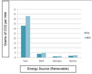
The two graphs compare the amount of CO2 given out (in grams) for every mile an electric vehicle and a non-electric vehicle need to travel. The first diagram compares non-renewable sources and the second, renewable. [8][9][10]
