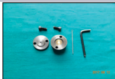
Figure 3: Prepared Light Cured Sample Mounted In Custom Designed Shear Punch Apparatus.
