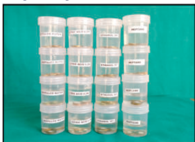
Figure-2: Prepared Samples Stored In Respective Dietary Solvents For A Week
