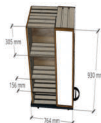
Figure 1: (D1) Street Crate Cart Structural Dimensions- 764× 502× 930 mm (length× breadth× height)
