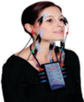
Fig. 3 – Surface EMG electrodes positioned on muscle fibres
