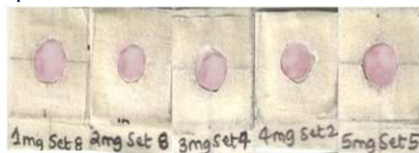
Fig 1. Optimisation of Substrate concentration (From left to right: Devices inoculated with substrate concentration ranging from 1-5 \text{gL}^{-1} )
