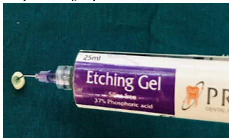
Fig:4 Group 1: sample treated using Acid etch
