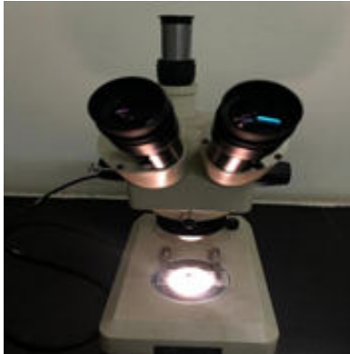
Fig 11: Stereo microscopic examination under magnifications of 2.5* 10× for microleakage observations
