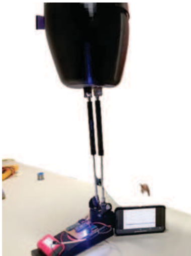
Figure 4: Actual Leg Connected With Mobile Phone To Track The Walking Pattern
