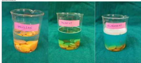
Fig-4 : Specimens Immersed In Respective Denture Cleansers
