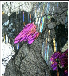
Figure 7: Photomicrograph of marble from Kelwa, Rajsamand, showing medium to coarse grained, inequigranular granoblastic texture. Carbonate grains (calcite and dolomite) are the major constituents. Impurities of muscovite are visible.
