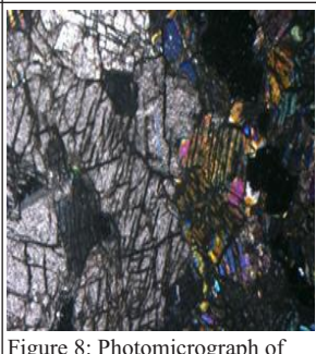
Figure 8: Photomicrograph of marble from Nijharna, Rajsamand, showing coarse grained, granoblastic texture. Carbonate grains (calcite and dolomite) showing well developed cleavages. Amorphibole is invariably present as accessory mineral.
