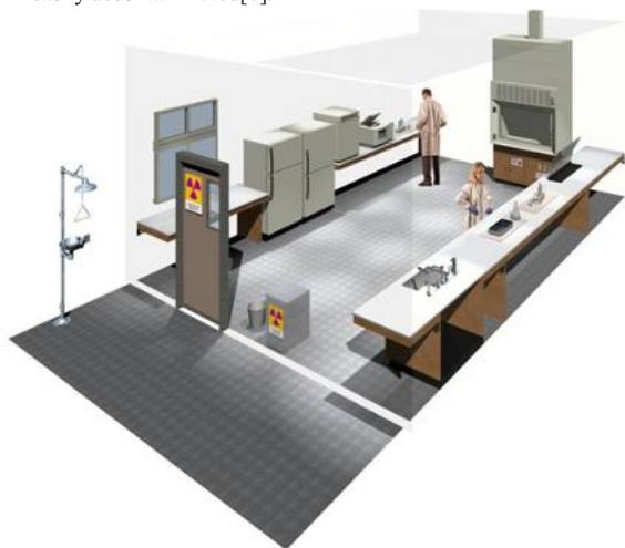
FIGURE 2: BIOSAFETY LABORATORY LEVEL 1 [NCB 1] IMAGE SOURCE: LABORATORY BIOSAFETY MANUAL , 3 rd EDITION, WHO; 2005
