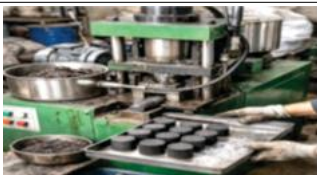
Fig. 1 Preparation of AFR Briquettes by Hydraulic Briquetting Press Machine
