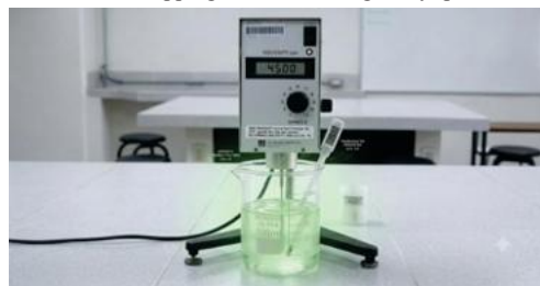
Fig 9 Viscosity Determination by Brookfield Viscometer
