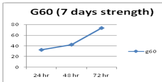
Figure 14 Oven Curing on Geo-polymer Concrete
