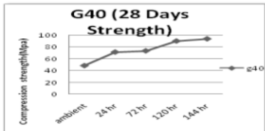
Figure 11 Showing Oven Curing on Geo-polymer Concrete for G40
