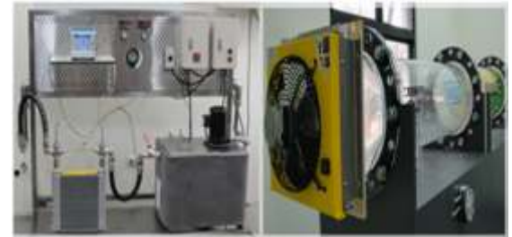
Fig.8 Cooler leak and performances testing
