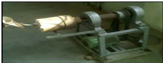
Figure 1. Horizontal Centrifugal Casting Machine Setup
