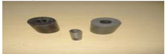
Fig 9: Die and Punch for P/M Process (1) is a oil hardened die and
