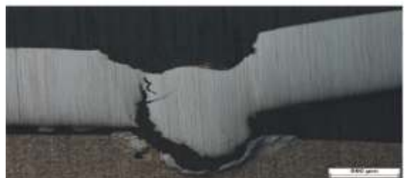
Fig. 7 Break of the welding seam within the steel sheet [6]
