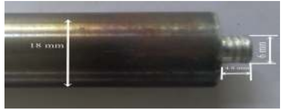
Fig. 6 Snapshot of the cylindrical threaded tool after welding [4]
