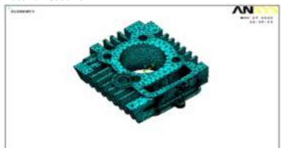
Fig.4. Meshed model of cylinder fin (2.5mm thick) body.
