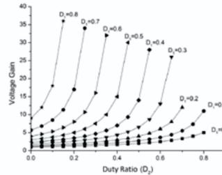
**Figure 5: Voltage gain corresponding to variations in duty ratio D1 and D2 for the proposed converter**
