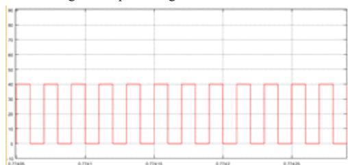
**Figure 8: Voltage across the switch of conventional boost converter**
