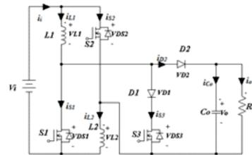
Figure 1: Proposed high gain converter
