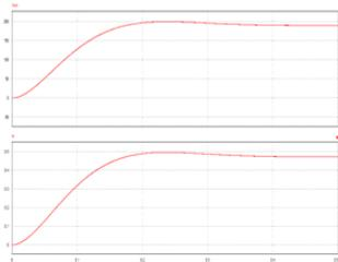
**Figure 11: Output voltage and current of the proposed converter**
