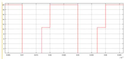
**Figure 13: Voltage stress across the diode of the proposed converter**
