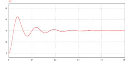
**Figure 7: Output voltage of conventional boost converter**
