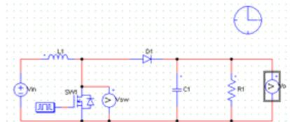
**Figure 6. Simulation diagram for conventional boost converter**
