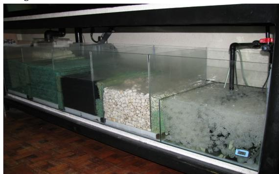
**Fig 1- Moving Bed Biofilm Reactor experimental setup**
