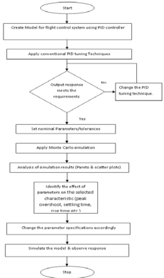
Figure.5 Controller Design using Statistical methods
