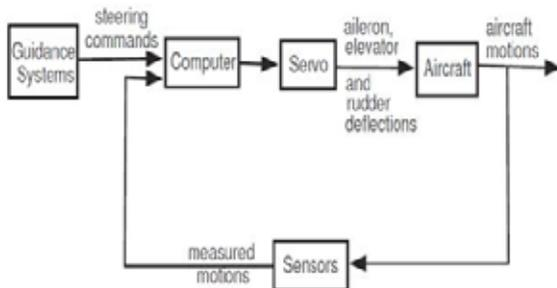
Figure 1. general closed loop control system for flight controls
