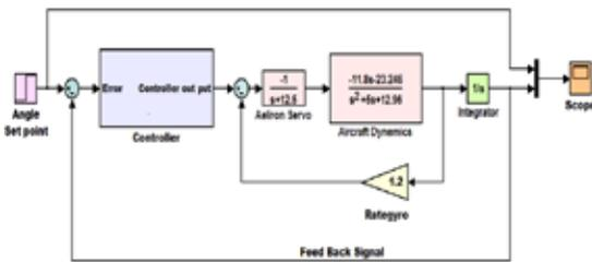
Figure.3 MATLAB/Simulink model for the system designed with Ziegler-Nicholas PID controller
