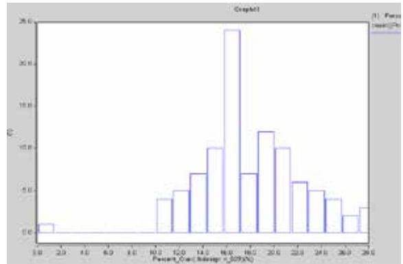
Figure.13 no of occurrences of overshoot value (after modification of tolerance range)
