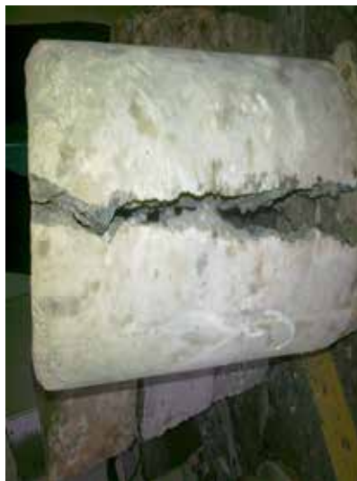
Figure 1: Failure of cylinders
