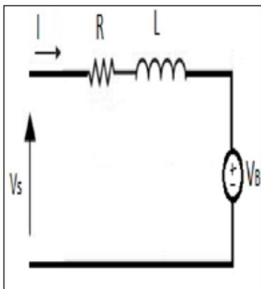
**Fig 2 Equivalent Circuit of DC Rotating Machine**
