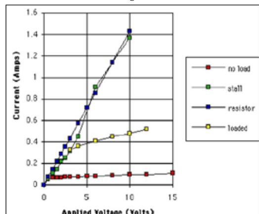
**Fig 1 Relationship between Machine Current and voltage**
