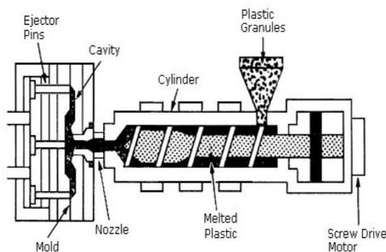
Fig. 1. Plastic Injection Molding Machine
