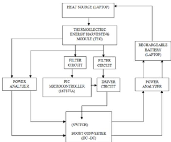
Fig 5: Block Diagram of Thermoelectric Energy Harvesting Module
