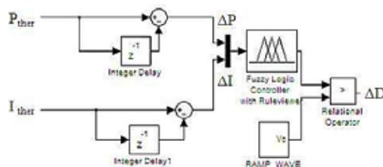
Fig 2: Block diagram of MPPT controller with modified hill climbing FLC method.
