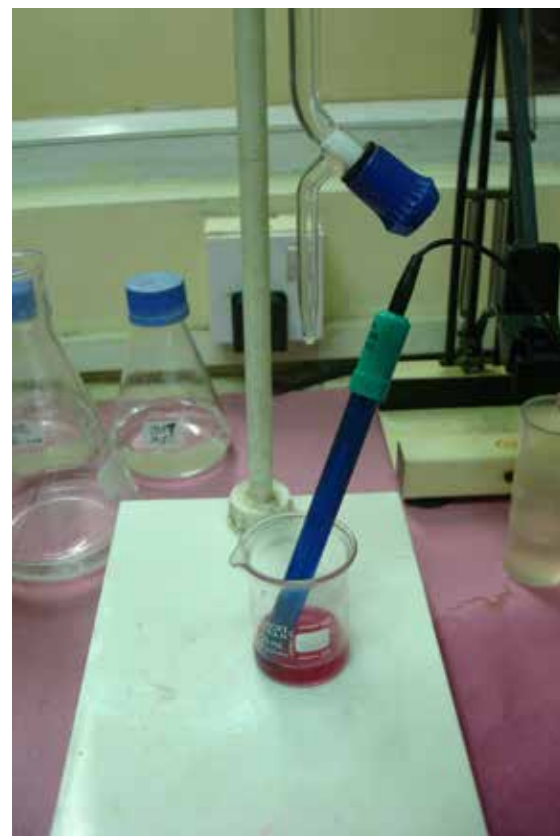
Figure 3: Measuring Titratable Acidity of different mouthrinses used in the study
