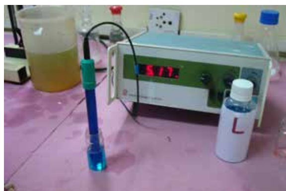
Figure 2: Measuring Endogenous pH of different mouthrinses used in the study
