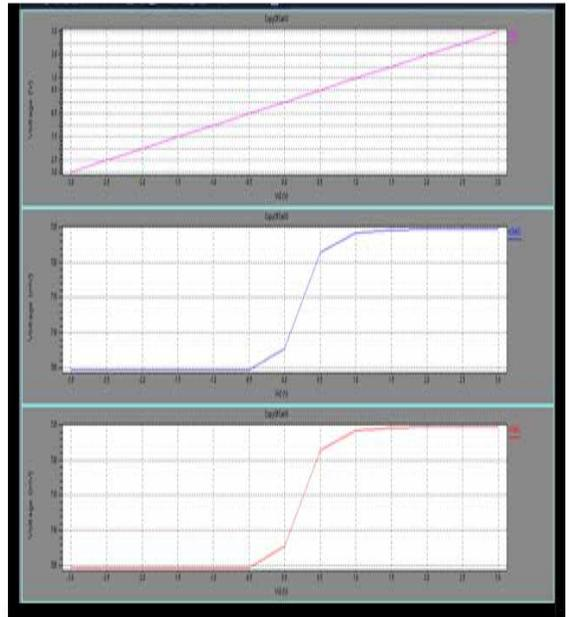
Figure. c. DC response obtained in common mode
