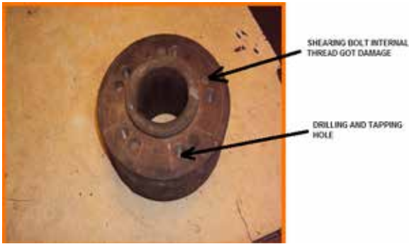
Figure6: New holes are drilled along the pitch circle diameter beside of old once
