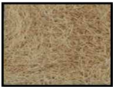
Plate 5: 100% Banana nonwoven fabric of 466 GSM (Cross laid)
