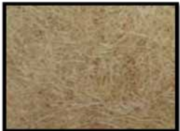
Plate 5: 100% Banana nonwoven fabric of 466 GSM (Cross laid)
