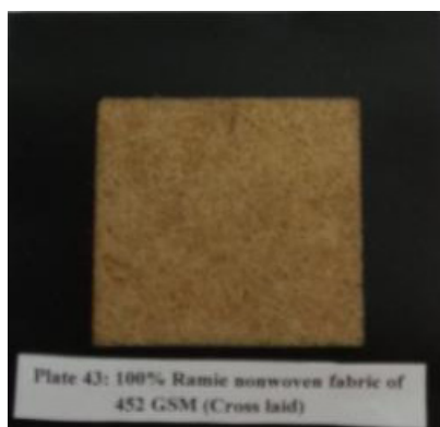
Plate 3: 100% ramie nonwoven fabric of 452 GSM (Cross laid)
