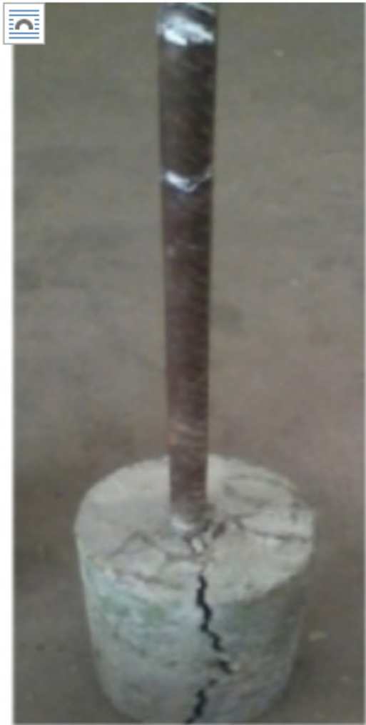
Figure-3 shows Failure pattern of cylindrical specimen in pull-out test.
