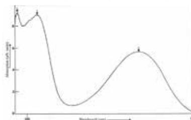
Fig. (a) UV- Visible absorption spectra of PANI without any metal doping
