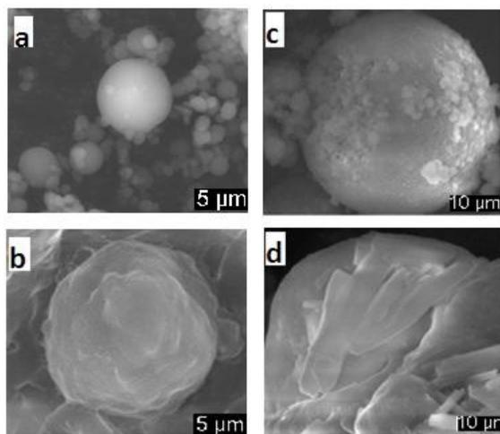
**Figure 4** Comparative SEM images of a) Normal PVC-emulsion grade b) Normal PVC-suspension grade c) Dechlorinated PVC-emulsion grade and d) Dechlorinated PVC-suspension grade
