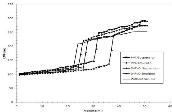
**Figure 2** Potentiometric titration graph (emf vs volume) of normal and dechlorinated poly (vinyl chloride) for determination of chlorine content.
