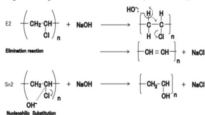
Scheme 1 Elimination and Nucleophilic mechanisms of Substitution reaction of poly(vinyl chloride) in NaOH solution.
