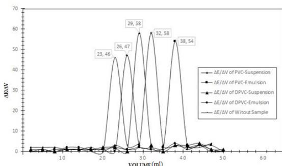
**Figure 3** Potentiometric titration graph (Change in emf vs volume) of normal and dechlorinated poly (vinyl chloride) for determination of chlorine content.
