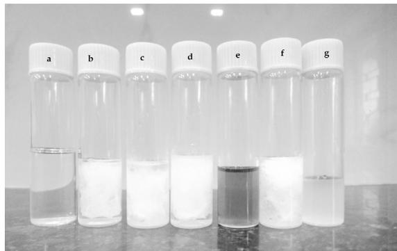
**Figure 6 Dissolution and precipitation test comparison a) THF and Water, b) PVC-S in THF but not in the Water) PVC-E in THF but not in water, d) DPVC-S in THF but not in water, e) DPVC-S (THF) and DPVC-S (water), f) DPVC-E (THF) and water and g) DPVC-E (THF)**
