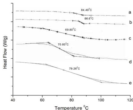
**Figure 5 DSC thermograph comparing the change in glass transition temperature a)suspension PVC, b)emulsion PVC, c)poly(vinyl alcohol) and d)dechlorinated PVC**
