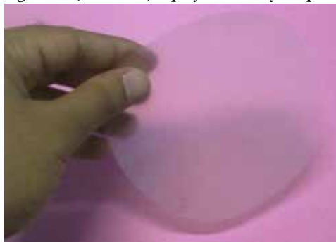
Figure 1: P(VDF-TrFE) copolymer film by hot press method
