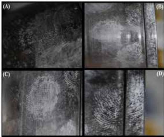
Figure 2 (A), (B), (C) & (D) shows the photographs of latent fingerprints developed on stainless steel bowl by cyanoacrylate fuming technique
