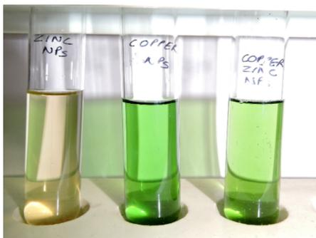
**Figure 1: Synthesized Zn NPs. Cu NPs., and Cu-Zn NPs. (from left to right)**
