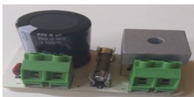
Figure 1: Rectified source 127 volts
