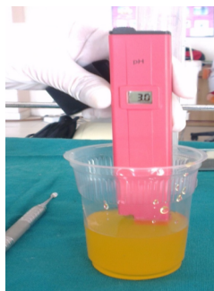
Fig 4: Endogenous pH measurement
