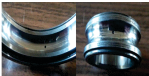
Figure 3: Artificial defects on the bearing components
